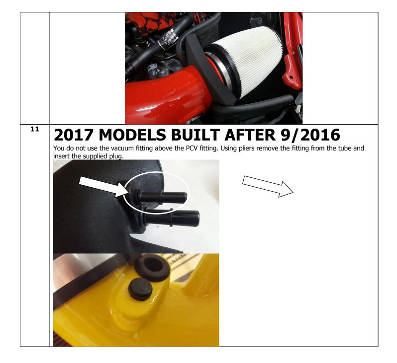
If not using the sound tube, remove factory tube all the way to the firewall and plug hole with supplied plug.
