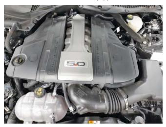
4. Remove the plastic caps exposing the fasteners holding the cover down. Unbolt the cover and pull up to remove it from the grommets.
