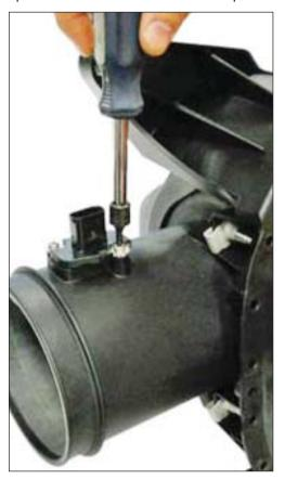
14. Install the lid onto the airbox assembly (P/N: 1318-9643HC-AA) Use six (6) self tapping screws (P/N: W506976-S437) to secure the lid.
