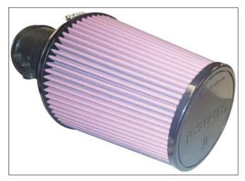
Slide the filter tube assembly into the air box (P/N: 131550-9A612), making sure the sensor boss is pointed toward the front of the vehicle. Using a 10 mm socket, install the two (2) bolts (P/N: W500224). Torque to 10 Nm. Rotate the air filter clamp to a suitable location and torque to 3 Nm.
