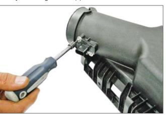
13. Re-install the MAF sensor into the ROUSH filter tube (P/N: 131550-12B579). Reattach the connector. Torque screws to 2 Nm.
