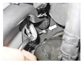
14. Using a trim tool, pry up on the push pin retaining the induction resonance tube and remove the tube from the vehicle.
