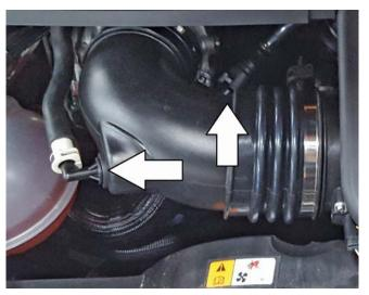
12. Remove the MAF sensor from the factory air box by removing the two (2) T-15 torx screws.
