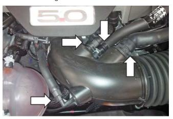
Using a 10 mm wrench or deep-well socket, remove the nut retaining the induction resonance tube to the firewall behind the driver side cylinder head.
