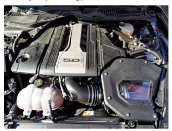
Re-install the engine cover and strut tower brace.
