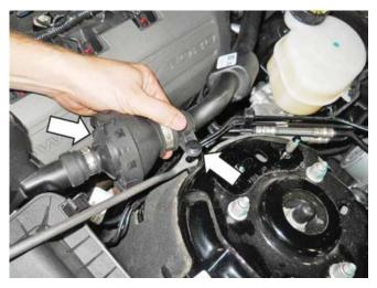
15. Remove the steel bushing followed by the two (2) rubber grommet from the stock air box tray. Retain these for use during installation.
