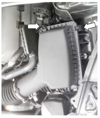
8. Remove the air box lid and filter. Retain the lid for use during installation.
