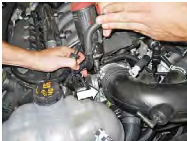
Clamp at throttle body
