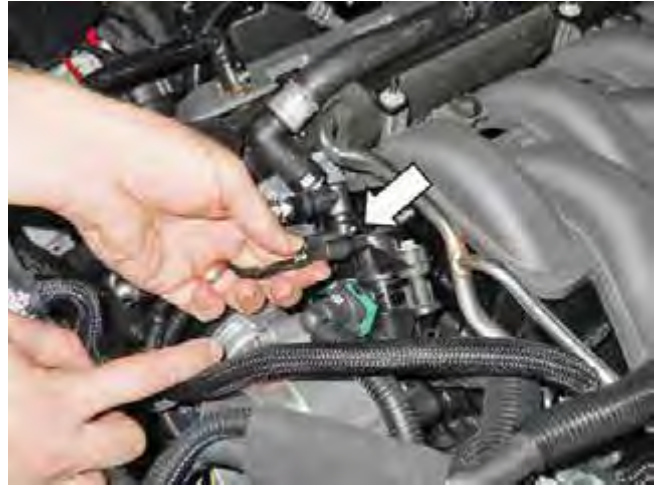
EECPV electrical connector
