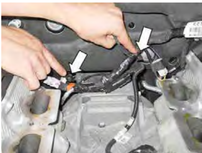
Pin retainers on harness
