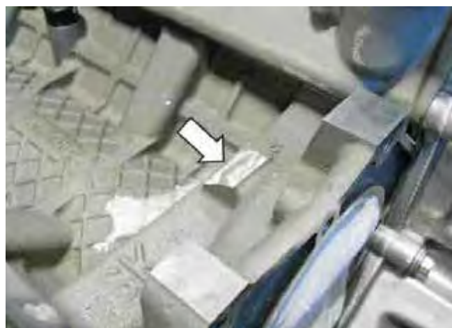
Grind area if intake won't seat
