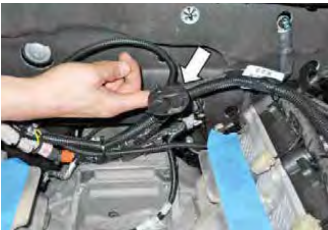
CMCV connectors taped up
