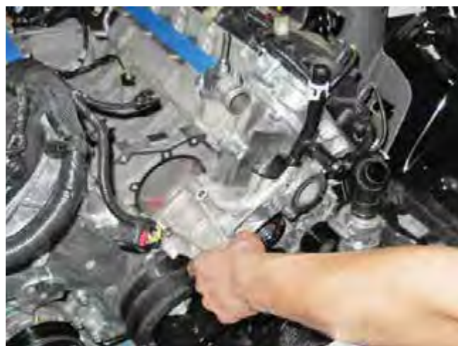
58. Place a clean towel in the water pump inlet cavity.
