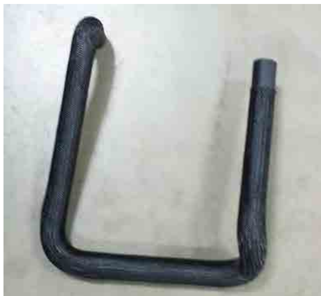
Intercooler pump outlet hose (1315-6K236)
