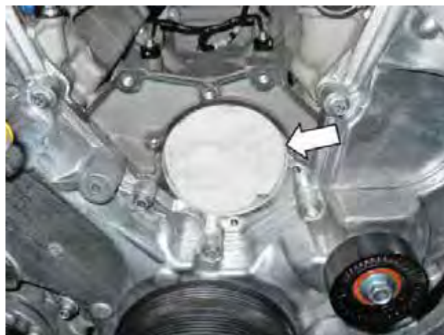
58. Place a clean towel in the water pump inlet cavity.
